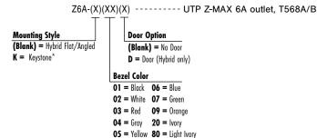
Each Z-MAX 6A UTP hybrid flat/angled outlet includes 1 printed icon set with the following color/print options.
